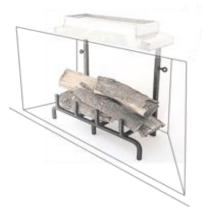
Visibly inspect that the **HearthCAT™** hood is flush against the back wall of the fireplace. If there is a gap of more than ½", then the smoke deflector must be installed in the back of the hood. Refer to the "Installation of the Smoke Deflector".
